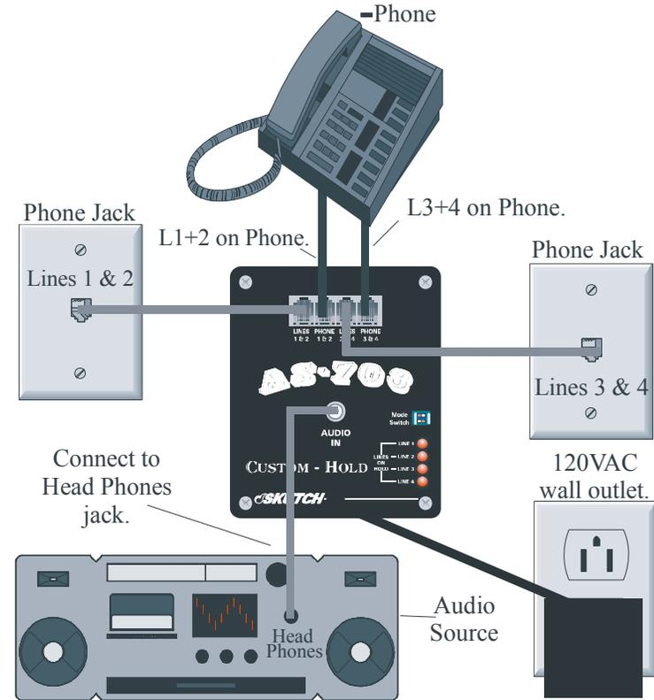
When a line is placed "ON HOLD", the corresponding LED on the AS-703-H will light indicating that audio is being coupled to that telephone line. The unit will play audio to all calls that are placed ON HOLD. Make sure that you adjust the level of the music to the proper level on the audio source.
